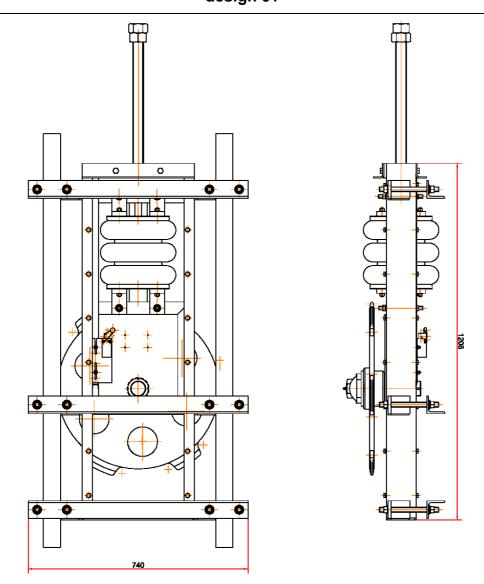
The tensioning device is used for all types of conveyers with zinc coated chain. It serves to the automatic tensing of the conveyer's chain. It eliminates influence on chain's wear and stretch trough the influence in operating and serves right chain tension during the whole life time of the chain.
